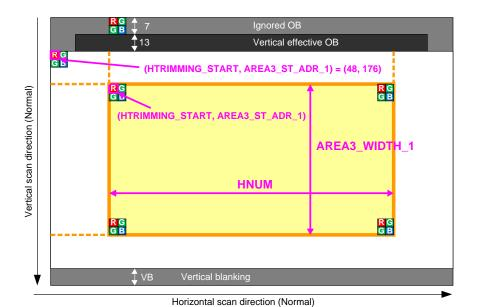
Image Drawing of Window Cropping Mode in normal vertical direction
