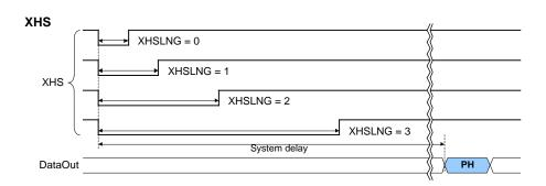
XVS/XHS output waveform in sensor master mode
