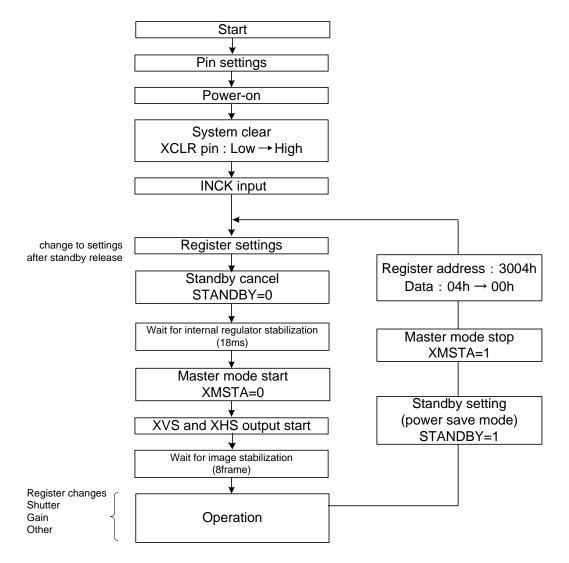
Sensor Setting Flow (Sensor Master Mode)
