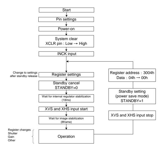
Sensor Setting Flow (Sensor Slave Mode)
