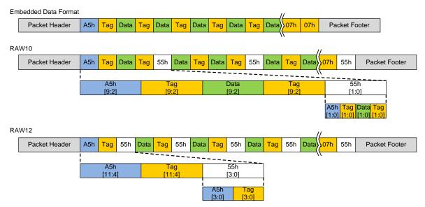
The end of the address and the register value is determined according to the tags embedded in the data.
