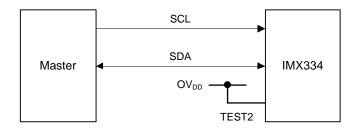
Pin connection of serial communication
