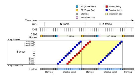
Image Drawing of Shutter Operation
