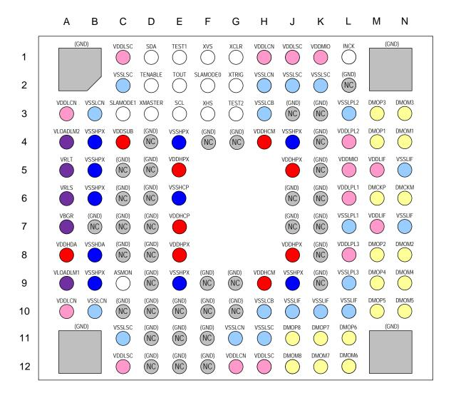
\*The N.C. pin can be connected to GND.
