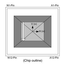
Normal and Inverted Drive Outline in Vertical Direction (TOP VIEW)
